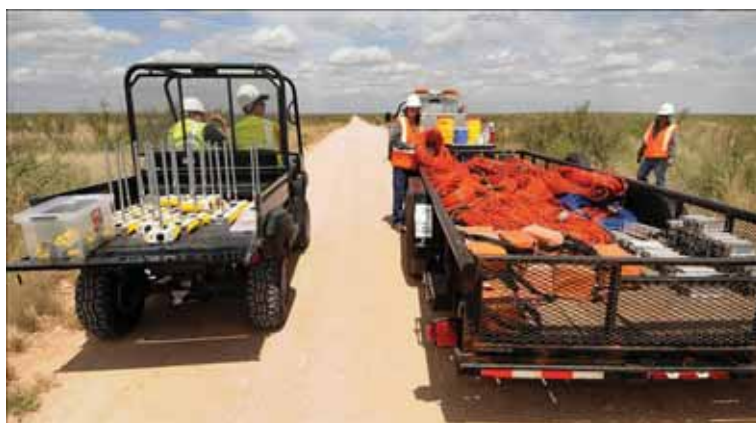
The wireless seismic equipment on the small truck on the left can do as many channels as the cabled equipment on the large truck on the right
