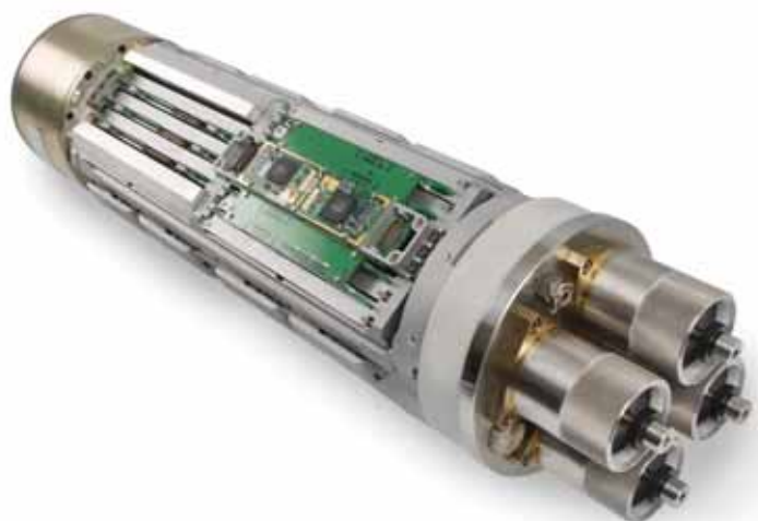
The Semstar5 subsea electronics module - GE has invested millions of pounds in the system, which can replace control systems on older equipment and give it a new lease of life
