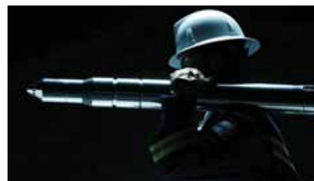
Wavefront's tool to add pulses to EOR fluid downhole
